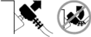
Figure 5-7 Disconnecting Defibrillation Cable from Test Post
