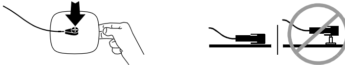
Figure 5-4 Connecting FAST-PATCH Electrodes to Defibrillation Cable
