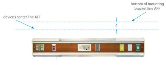
3. Using a stud locator, mark the location of any metal studs or blocking in the building wall that intersect the console mounting location.
