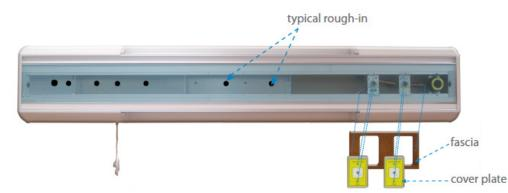
6. Hang the console unit on the wall, over the mounting bracket, and center the unit with reference to bed center line. Verify rough-in locations in wall and align with rough-in provisions on console.
