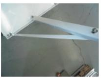
Repeat above step by setting the BT-FL-STAND-CROSSBAR diagonal to the BTFL-STAND-CROSSBAR inserted in the above step. This is shown below:
